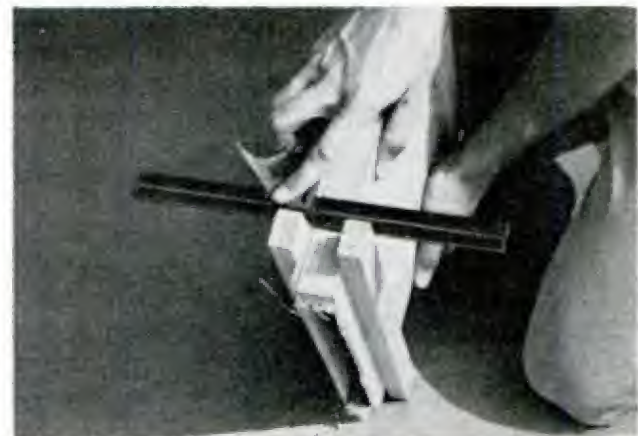
DAGGERBOARD TRUNK is fiberglassed inside before assembly. Below: Bed logs must be carefully aligned
